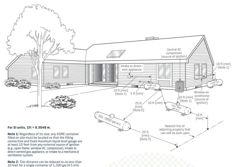
at least 25 feet from any other LP-gas container of more than 125 gal (0.5 m3) water capacity.
